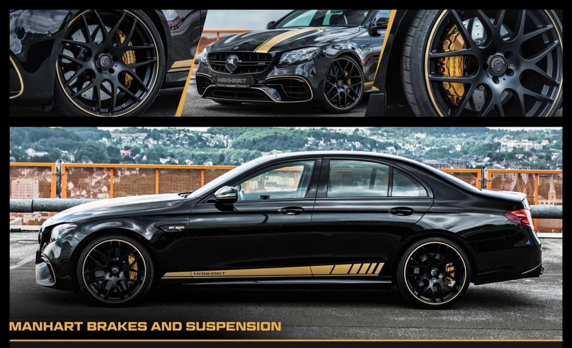
To ensure that the ER 800 not only accelerates much more rapidly than the basic E 63 S, but also comes to a stop again even more quickly, we have installed a ceramic brake kit with 405x38mm diameter discs on the front axle of the ER 800. With regards to lowering the factory air suspension by 20 to 30 millimeters, there are two different variants to choose from: either, as in the case of the example shown, by using new coupling rods or via a software adjustment.
