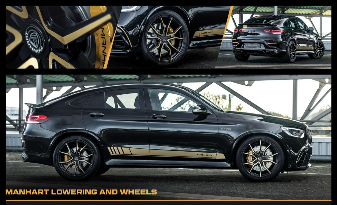
On the chassis side, we also upgraded the GLR 700: The car is about 30 millimetres lower, thanks to a revision of the standard air suspension with new coupling rods. Incidentally, the GLR 700 is instantly recognisable as a MANHART. After all, it stands on our Spider Line alloy wheels in 9×21 and 10.5×21 inches with tyres in 265/40ZR21 and 295/35ZR21. On the car shown, they have a satin black finish with gold rim decoration. Alternatively, any other desired configurations are also possible.
