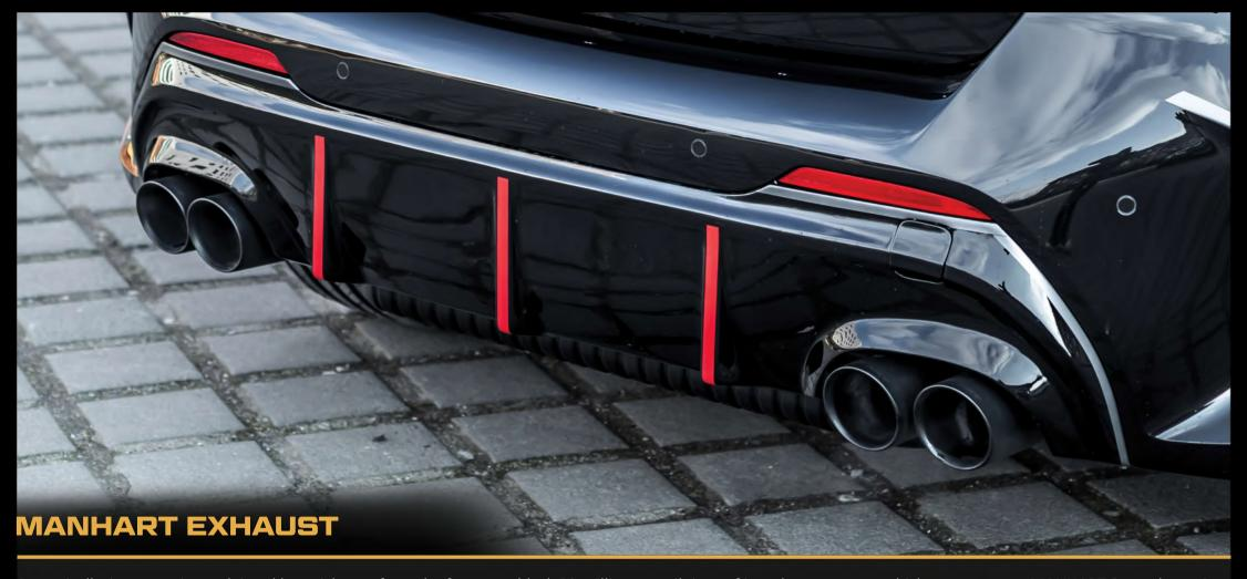
Acoustically, its power is proclaimed by a rich roar from the four matt black 90-millimeter tailpipes of its exhaust system, which connects to a MANHART Sport downpipe with a 300-cell HJS catalytic converter. The latter – like the optional OPF deleter including linkpipe – is not TÜV-approved and is therefore only intended for export.
