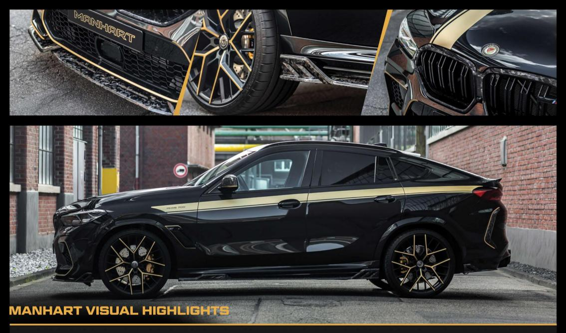
Visually, the MHX6 700 has also been extensively revised: For example, suspension optimisation and MANHART lowering by means of H&R springs have reduced ground clearance by 30 millimetres. MANHART Classic Line-Y-spoke rims provide the ground contact. They feature a satin black finish with coloured accents in gold, measure 10.5x22 inches and are fitted with 295/30R22 tyres.
