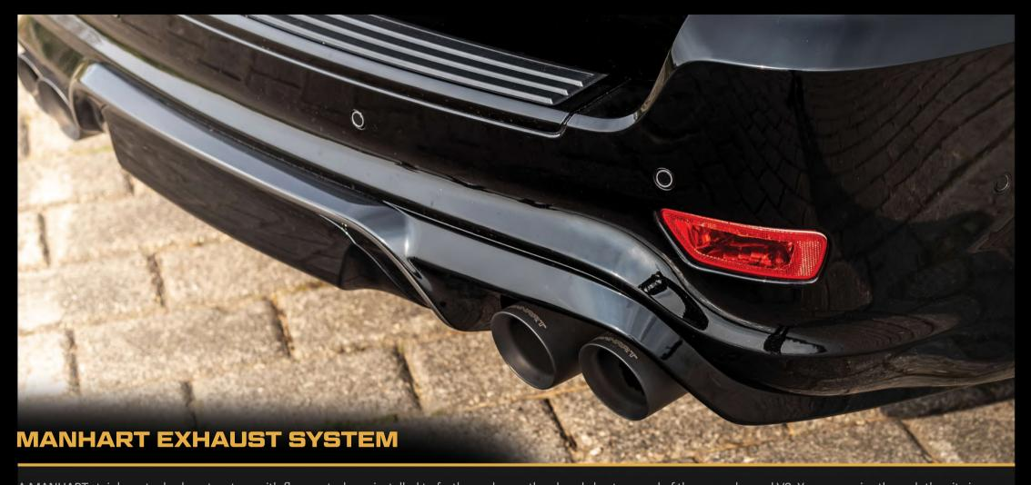
A MANHART stainless steel exhaust system with flap control was installed to further enhance the already brute sound of the supercharged V8. You can cruise through the city in peace and quiet or enjoy the wonderful sound of a 6.2-litre V8 in the right and powerful pitch when you need it. The sound is by no means unpleasant, but only much more powerful.
