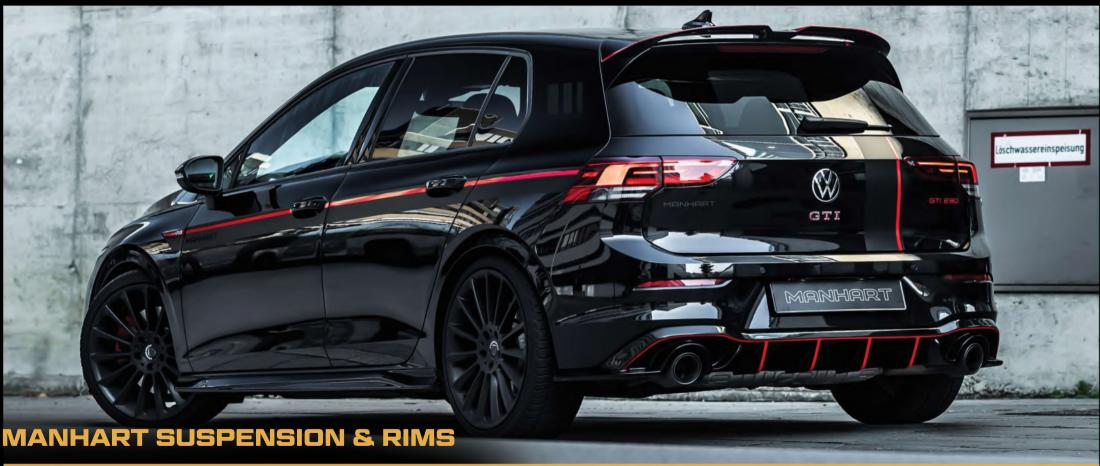
Essential, visual adjustments that give the car an even more coherent and dynamic appearance, are undoubtedly the new wheels and the lowering: The latter is due to a set of H&R springs, which lower the body by 40 millimetres. The MANHART multi-spoke rims in Venturi style mounted under the wings have the dimensions 8×19 inches ET40, the mounted tyres measure 225/35ZR19.
