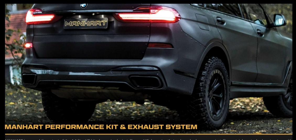
MANHART increased the output of the 4.4-liter V8 biturbo engine by installing an HJS downpipe that reduces back pressure, installing a stainless steel exhaust system with valve control and by optimizing the software from the standard 530 hp and 750 Nm to 650 hp and 920 Nm.
