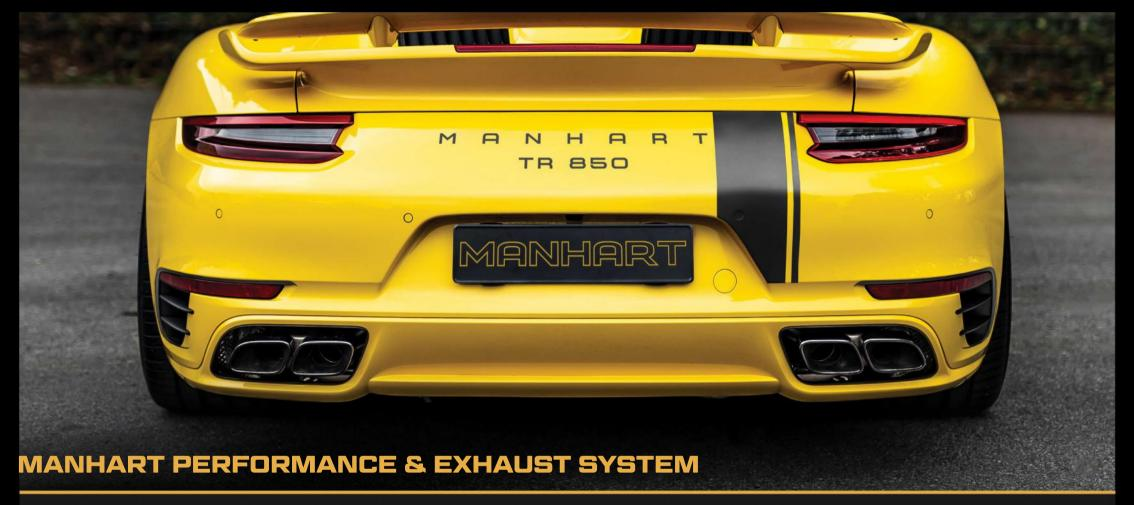
The 3.8-liter 6-cylinder engine was upgraded to 850 HP and stunning 1090 Nm. These staggering numbers are confirmed through the brutal sound the Turbo produces after the MANHART stainless steel exhaust system including muffler with flap control was fitted alongside a set of MANHART downpipes "Sport" with 200 cells HJS catalytic converters.
