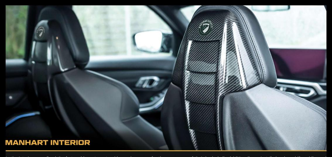
In the interior, we refined the factory M sports seats with a carbon cover for the upper area of their back shells. Additionally we installed carbon shift paddles and illuminated MANHART door sills.
