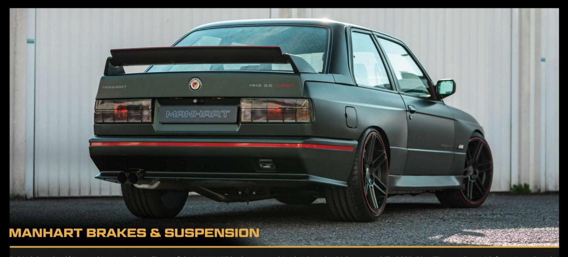
Behind the wheel/tire combinations, the callipers of the MANHART brake system shine bright red, which acts on drilled 330x32 millimetre discs with four-piston Brembo fixed callipers at the front. At the rear, also drilled brake discs were combined with the E30 M3's OEM floating callipers. A MANHART monotube coilover suspension by H&R ensures optimal road adhesion of the wheels and extremely agile handling of the civilian racing touring car.
